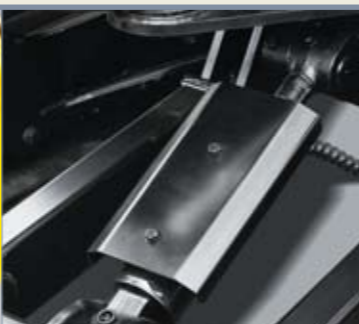
Dozer Cylinder Cover
