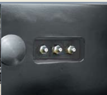
Centralized Grease Fittings
