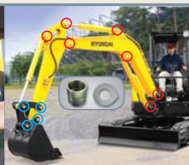
Low maintenance bushings and polymer shims
